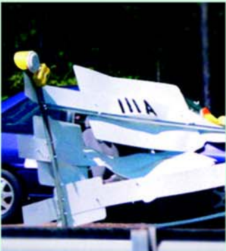
Type III barricade with ALPOLIC® 350 signs crash test
