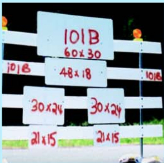
ALPOLIC® 350 signs and barricade prepared for testing to NCHRP 350 requirements
