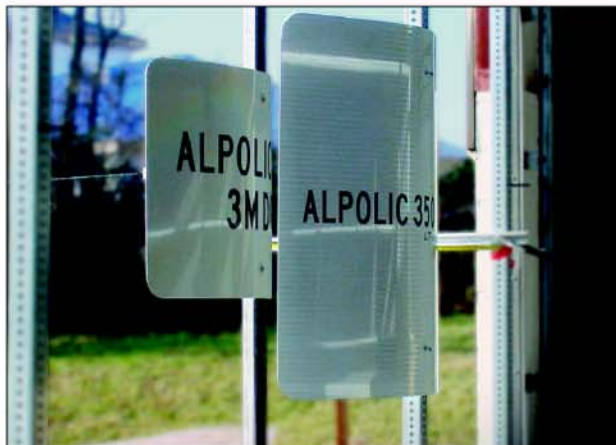
ALPOLIC® 350 was subjected to hurricane force wind testing at ATI
