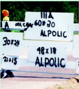
Type III barricade with sign blanks mounted for crash test
