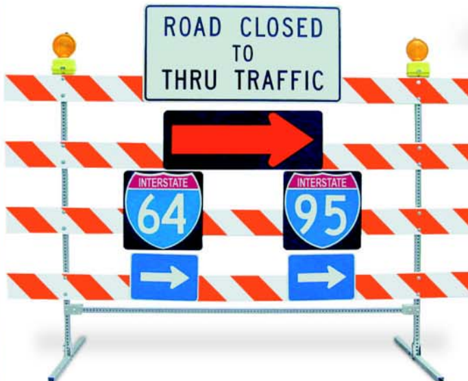
Type III barricade with sign blanks mounted for crash test
